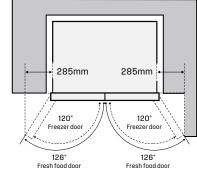
When positioned in a corner area, spacing of at least 285mm on the hinge side will allow the doors to open enough to enable the removal of bins and shelves.
