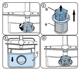
To remove and clean the filter combination, turn it counter clockwise and remove it by lifting it upwards (1). Pull the coarse filter out of the micro filter (2). Then pull and remove the metal filter (3). Rinse the filter with lots of water until it is free of residue. Reassemble the filters. Replace the filter insert, and rotate it clockwise (4).
