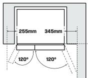
When positioned in a corner area, spacing of at least 345mm on the right hinge side and 255mm on the left hinge side will allow the doors to open enough to enable the removal of bins and shelves.
