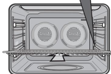
2. Drop the front of the shelf or tray onto the slide ensuring it sits behind the front post of the slide.
