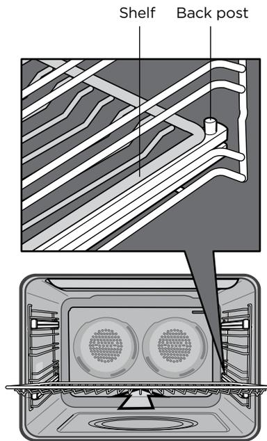
2. Drop the front of the shelf or tray onto the slide ensuring it sits behind the front post of the slide.
