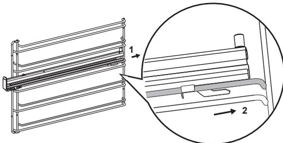
3. Push slide front clip over wire until secured.
