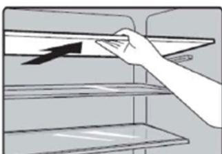
To replace, hold the shelf straight with the fridge cavity, angling the shelf downward. Slide the shelf in on the shelf runner, and gently drop into place.
