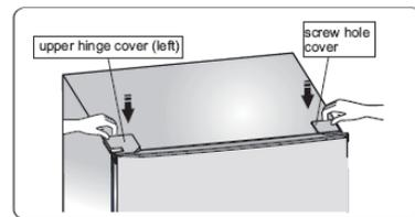
7. Replace part ③ to the left side and fixing it with the screws ④ . Replace part ① and part ② to another side and fixing it.
