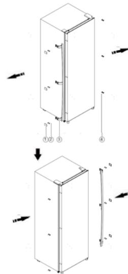
Note: 1. You need move hinge axis from hole ① to ② , move adjustable bottom feet part from hole ③ to ④ before transfer.
