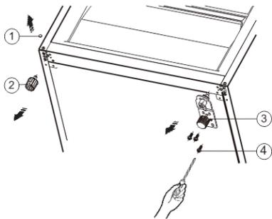
10. Put the screw hole cover and upper hinge cover (left) as follow diagram.
