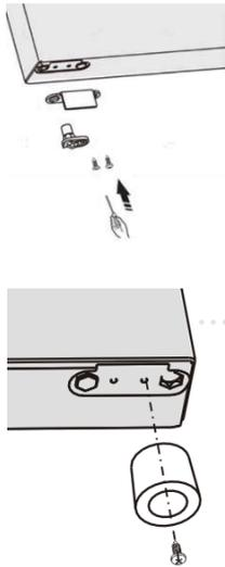
8. Set the door into its new place making sure the pin enters the bushing at the lower frame section.
