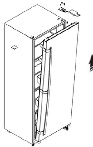
5. Loose screw ② and screws ⑤ , detach part ① and part ③ part ④ . Replace part ① to the right side and tighten securely with screw ② . Replace part ③ and part ④ to the left side and tighten securely with screws ⑤ .
