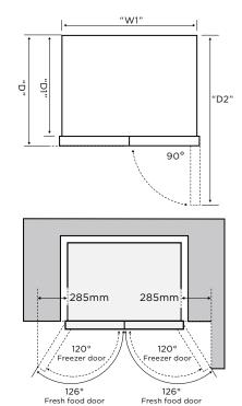
When positioned in a corner area, spacing of at least 285mm on the hinge side will allow the doors to open enough to enable the removal of bins and shelves.
