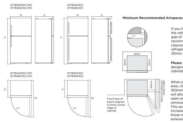
If you have a cupboard above the refrigerator with a rear gap of less than 100mm (Y), recommended minimum clearance at the top of the refrigerator increases from 30mm to 70mm (X).
