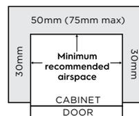
Please note: Doors are designed to sit proud of cabinetry (not flush). The clearances shown above are the recommended minimum clearances. The clearance at the rear must not exceed 75mm.
