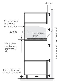
6mm packer Please note packer must be set back 20mm from front trim to avoid obstruction of front vent. Packer must be secured to base of cabinet.
