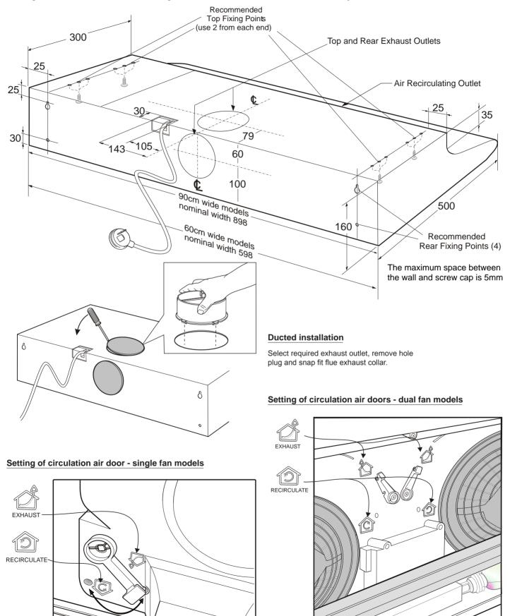
IMPORTANT: SET CIRCULATING MODES BEFORE INSTALLING THE HOLE PLUGS.
