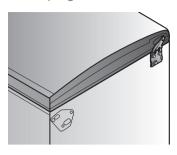
27. Clip the LH hinge cover (kit contents) over LH top hinge.
