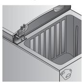
9. Remove RH centre hinge by lifting the door slightly and sliding hinge out of the door
