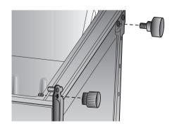
19. Replace the food door by holding at 45° and gently slide onto the
