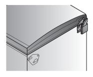
28. Insert the RH top hinge hole cap (kit contents) in the cabinet as
