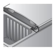
22. Replace the freezer door by holding at 45° and gently slide onto the centre hinge and closing the door.
