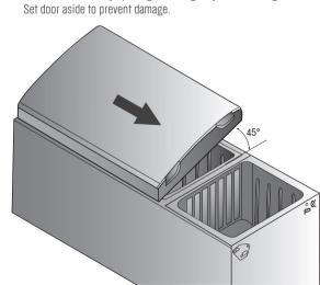
11. Remove both the nylon bearing and the nylon bearing cap from the top of door and swap positions. Repeat with freezer door. Remove RH door
