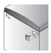
Unscrew 3 x 8mm top hinge screws and remove RH top hinge. Do not discard screws.
