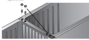
13. Unscrew the hinge foot using phillips head screwdriver and unscrew foot on opposite side. Do not discard.
