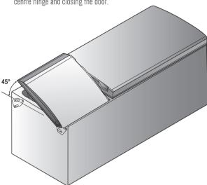
23. Slide the LH top hinge (kit contents) into the door, loosely screw the 3 x 8mm screws from the existing top hinge in the cabinet.
