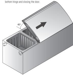
20. Replace LH centre hinge by lifting the door slightly and sliding hinge into the door and placing the door down again.
