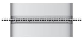
26. Fully tighten the LH top hinge to the cabinet until the hinge is secure.
